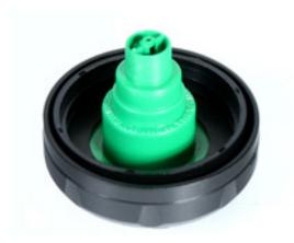
Above is the cap as it comes out of the package, or straight off your tank. Step one is to VERY CAREFULLY remove the rubber seal that holds that green part in (this is the vent body). Use a dull bladed screwdriver to GENTLY lift up the gasket until you can grasp it with your fingers.
