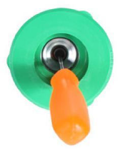
The image above shows the pick tool stuck in the gasket at the bottom of the vent body. You just want to poke a hole in this small rubber piece. Do not cut it or mutilate it or remove it. Any of those things will cause fuel to possible spill when the tank is full or when the bike is tipped over.
