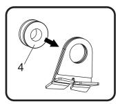
5. Install (No. 5) *ALS-046*, aluminum spacer in the front side of (No. 4) *Z1023*, rubber grommet and install (No. 6) *ALS-054*, aluminum spacer in the back side of (No. 4) *Z1023*, rubber grommet as shown below.
