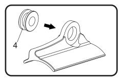
7. Install (No. 7) *ALS-047*, aluminum spacer in the backside of (No. 4) *Z1023*, rubber grommet and install (No. 5) ALS-046, aluminum spacer in the frontside as shown below.
