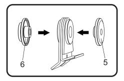
6. Install (No. 4) *Z1023*, rubber grommet into muffler bracket.
